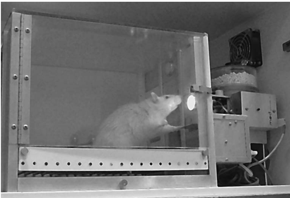
Figure 1.1 An experimental chamber in which a rat can receive food pellets by pressing a lever.
